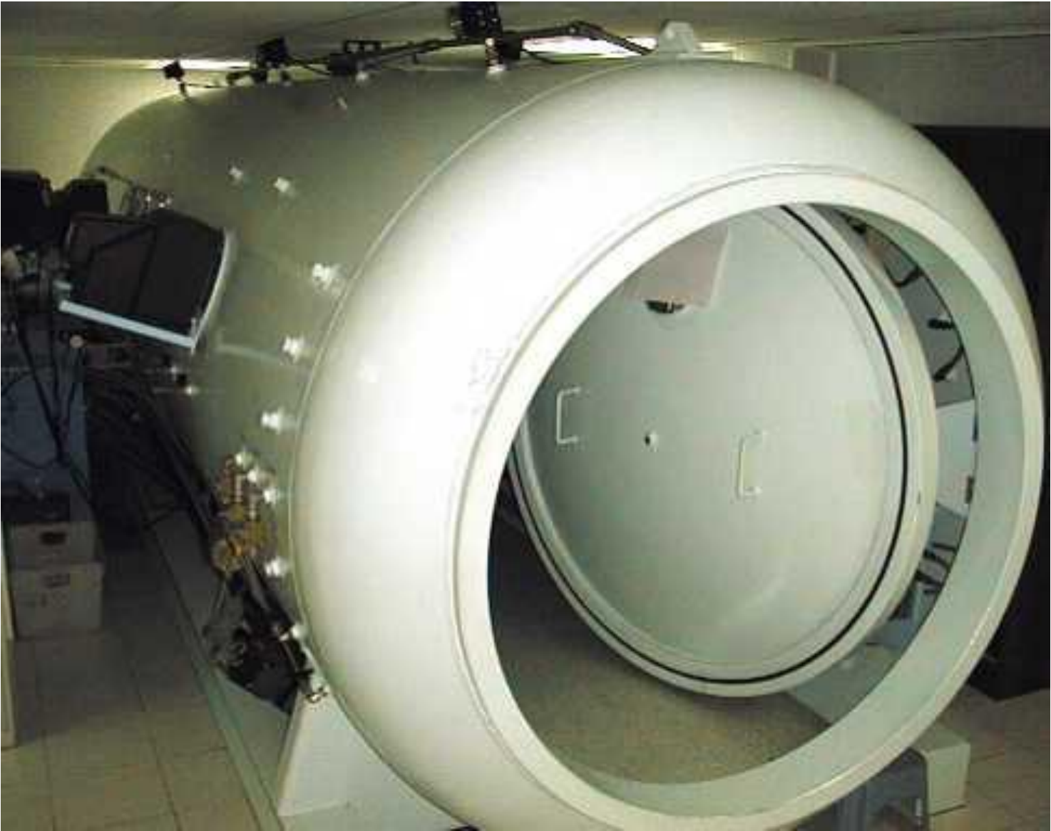
Patient Entry Door to Main Treatment Lock
