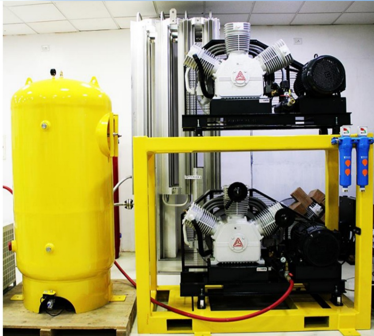
Reciprocating type, oil-free compressors (2 units), air dryer and air receiver
